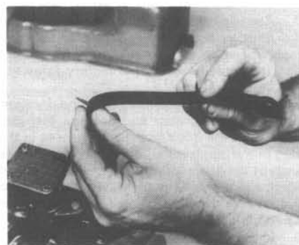
34.4 During installation the rubber tips on the front oil pan gasket should be pressed into the holes in the timing gear cover
