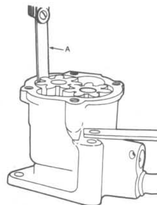
Fig. 2.31 Checking the oil pump gear-to-body clearance with a feeler gauge (Sec 60)
