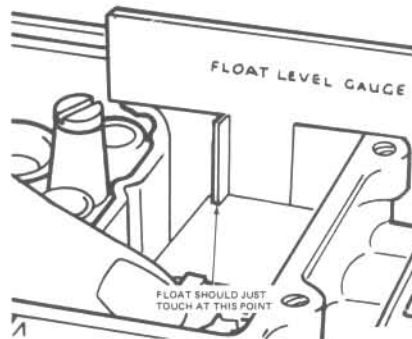
Fig. 4.31 Measuring the dry float level (2100/2150 carburetor) (Sec 13)
