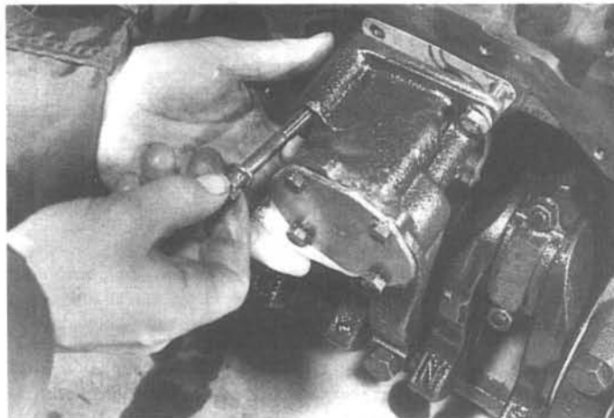
66.2 Installing the oil pump
