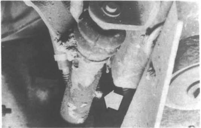
7.8 Clutch lever shaft grease fitting location (arrow)
