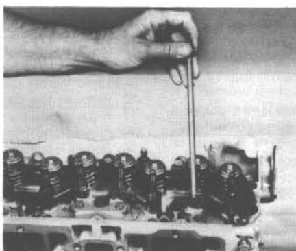
29.12 Removing the pushrods
