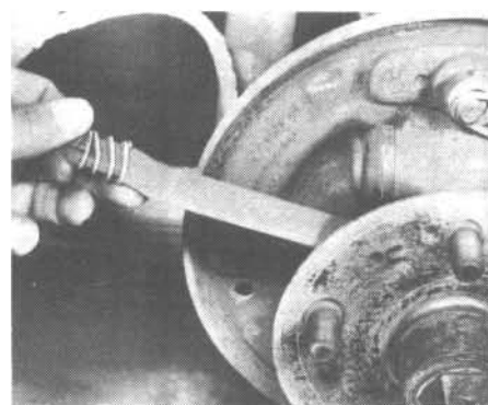
12.9A Removing the rear brake parking brake strut
