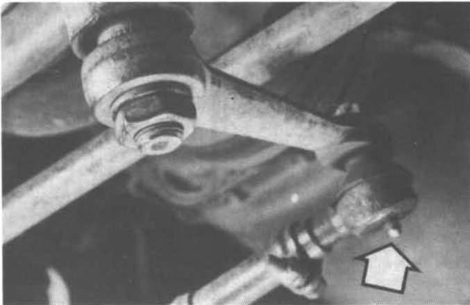
7.2 Steering arm grease fitting location (arrow)
