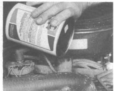
5.24 Pouring oil into the filler opening (V8 engine shown)
