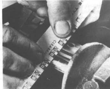
19.14 The crushed Plastigage is compared to the scale printed on the container to obtain the bearing oil clearance
