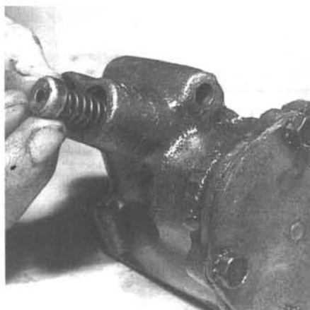
60.7B Insert the spring retainer
