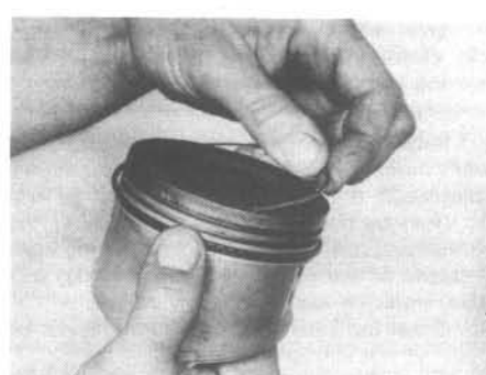
18.9B Do not use a piston ring tool when installing the oil ring side rails
