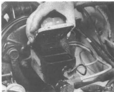
4.24 Checking the brake master cylinder fluid level
