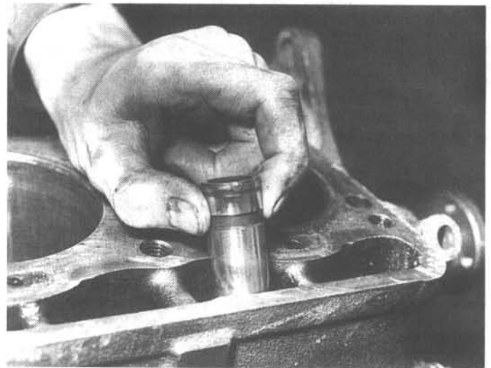
49.3 Removing a valve lifter
