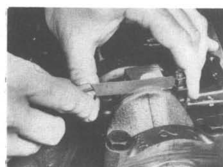
11.6 Checking connecting rod end play with a feeler gauge
