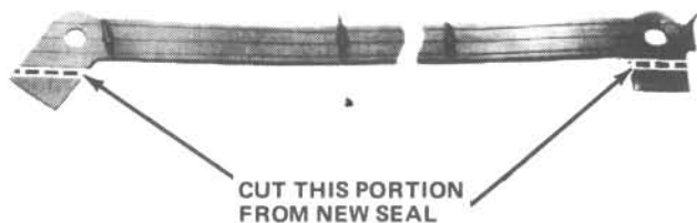
Fig. 2.19 The front oil pan gasket must be cut as shown to form a proper seal with the side gaskets (Sec 34)
